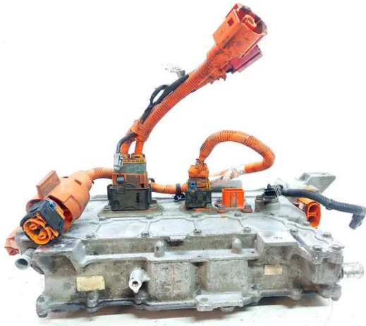
Inverter or Variable Frequency Drive
